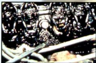
Commercial grade oil after 21,000 miles in severe police car service.
